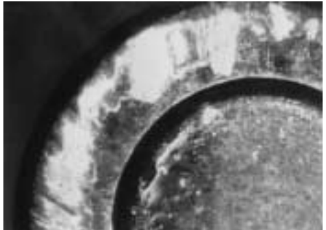
Fig. 15-4 Scratches on Larger Side Surface of Tapered Roller Bearing
